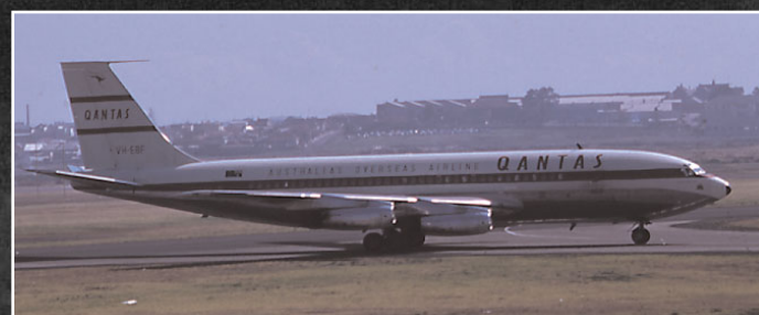
Above: Colour shots of the Qantas 707-138s in their original form and colour scheme are rare. This one shows VH-EBF at Sydney's Mascot Airport in August 1961, just four months before it was converted to turbofan engines as a 707-138B.
